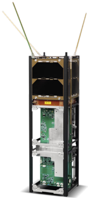
SpooQy-1: Singapore's experimental quantum CubeSat for testing a source of entangled pairs of photons.
