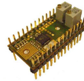
Figure 1: HG2M Package (DIL28)
