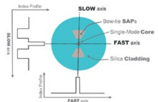
Typical 'Bow-Tie' HiBi Fiber Geometry
