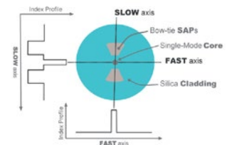
Typical 'Bow-Tie' HiBi Fiber Geometry
